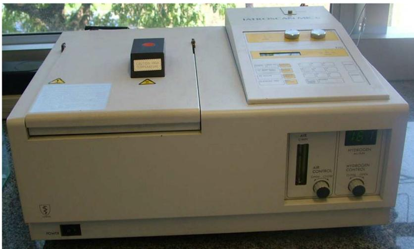
Figura 5.6 - Analisador de TLC-FID (Thin Layer Chromatography – FID) (Iatroscan).
