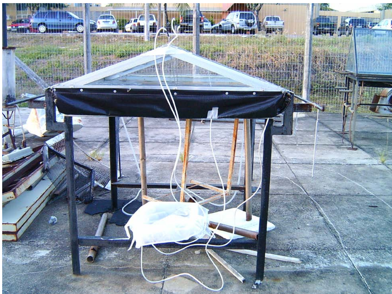
Figure 1. Photograph of the solar still used in this work.
