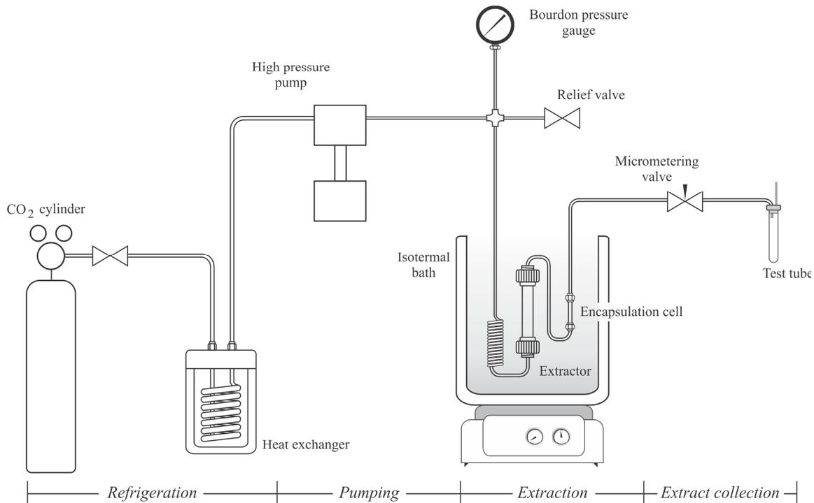
**Figure 2.** Experimental apparatus that was used for extraction and encapsulation.
