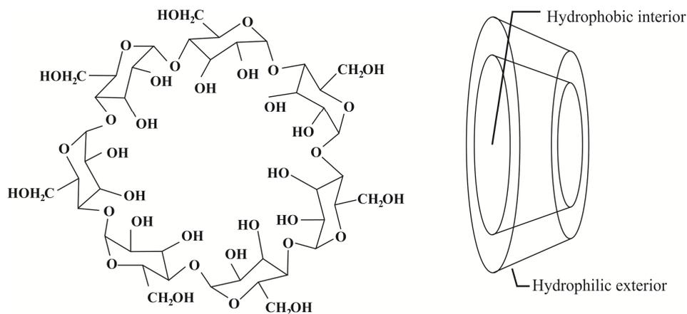
**Figure 1.** Molecular structure of  $\beta$ -cyclodextrin
