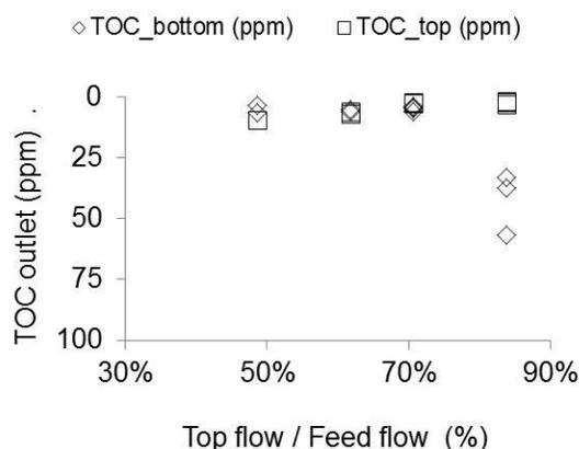
Figure 3. Values of TOC in the top and bottom effluent as a function of the upper effluent fraction at injection temperature of 20°C and 13.5% of IPA
