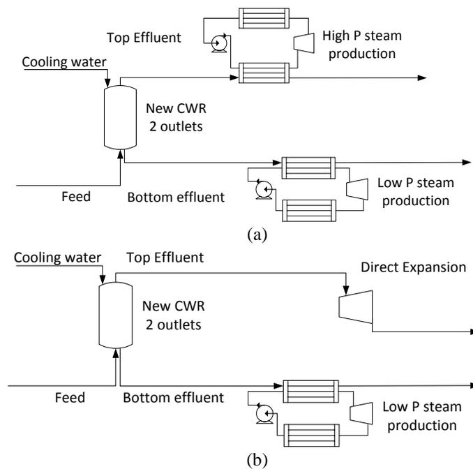
**Figure 4.** Scheme of the different options for the recovery energy with the CWR with 2 outlets (a) Steam production, (b) direct expansion of top effluent
