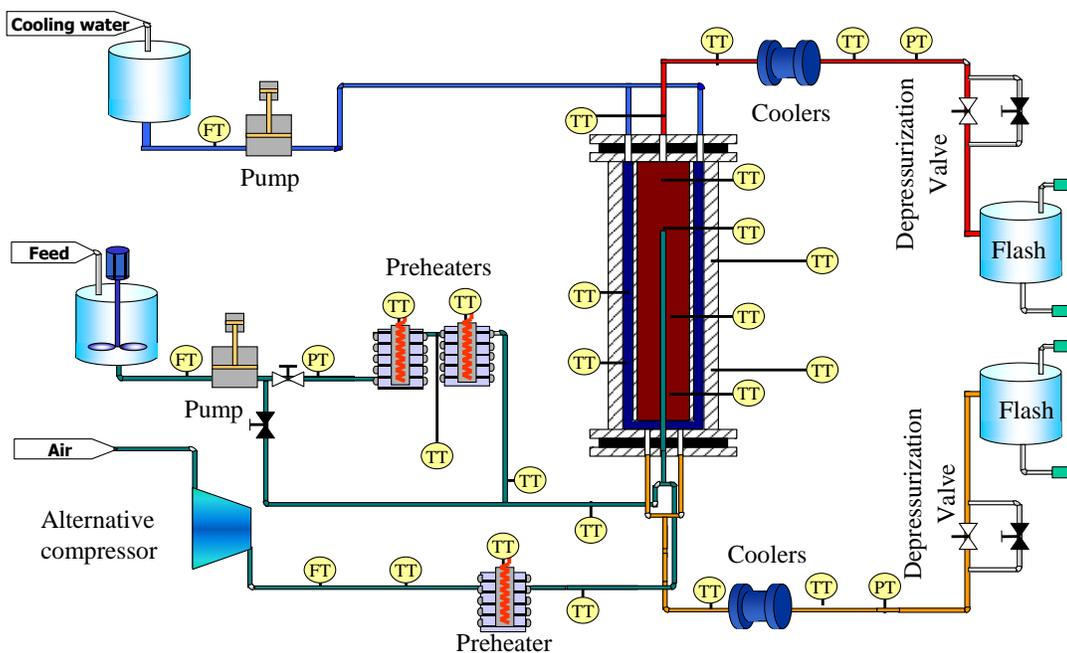
Figure 1. Diagram of SCWO facility with two outlets.
