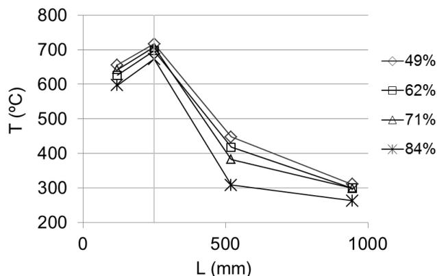
Figure 2. Temperature profiles for different upper effluent fraction at 20°C
