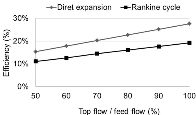
**Figure 5.** Efficiency of the recovery energy of the new reactor with (a) direct expansion and (b) steam production
